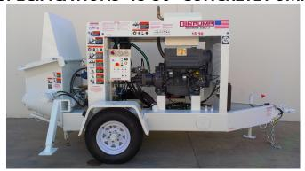
28/35 OUTPUT: cmh/cyh **DELIVERY PRESSURE:** bar/psi 53/750 **DELIVERY CYLINDER: mm/inch** 127/5 STROKE: mm/inch 610/24 **STROKES/MINUTE:** 60 36/48 **ENGINE POWER: kw/hp** HOPPER CAPACITY: I/gal 299/79 **OUTLET:** mm/inch 127/5
