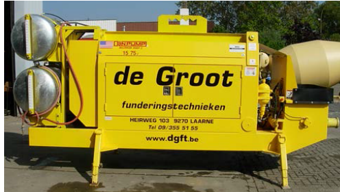
LEG MOUNTED UNIT SHOWN W/ NOISE REDUCTION ENCLOSURE
